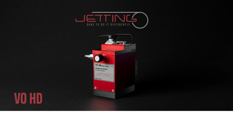
Extremely compact electrically operated fiber blowing machine optimized for FTTX installation of blown fiber (EPFU) and micro/nano cables, from 0,8 to 6,5 mm into duct from 3 to 16 mm.
